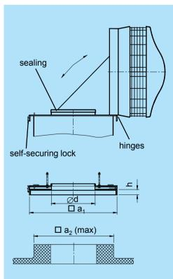
The hinged roof upstand is used if fast access to the ventilation duct or to the fan is necessary, such as for maintenance or duct cleaning. Two profiled plastic plates are connected by hinges and tensioned by self-securing locks. A protective device keeps the open fan safely in position. A profiled seal ensures tight connection to the duct and prevents from soaking of rain water.
