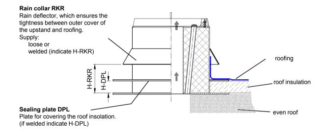
Installation on foundations (upstand preferably with rain water edge)
